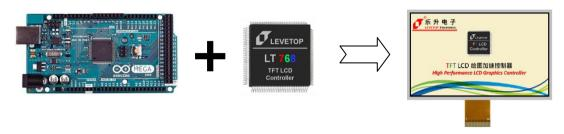
To help Arduino users develop projects with the TFT display using LT768x (LT7681/LT7683/LT7686) controller, Levetop provides a complete library for Arduino platform. This manual is to illustrate how users can setup and apply such library in their projects, based on Arduino Mega2560 board. For more information about LT768x controller, please refer to LT768x datasheet and the application note.
